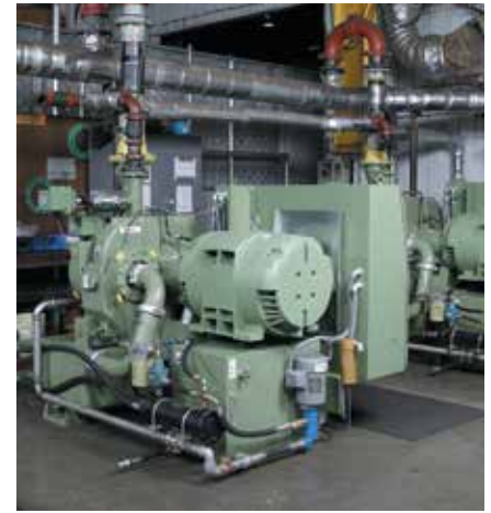
Standard package test of TURBO-AIR 2000 in Cameron's test center.
