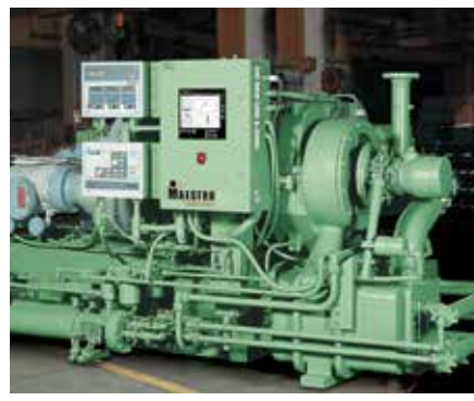
One 375 kW (500 hp) TURBO-AIR compressor in compliance with API 672 for an oil refinery.
